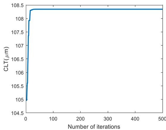
Figure 3: Convergence curve of CLT using TLBO algorithm
