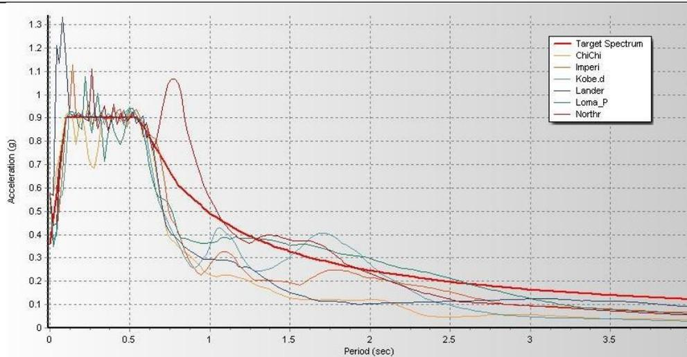
Fig. 5 - Scaled acceleration time histories of considered earthquakes
