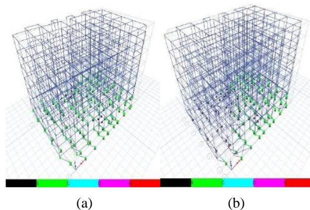
Fig. 16 - Hinge failure pattern for: (a) Base Model (b) Retrofitted Model
