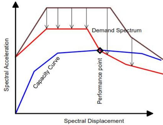
Fig. 8 - Performance based design approach (Kiran et al, 2017)
