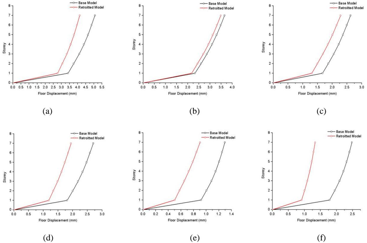
Fig. 12 - Observed values of Storey Displacement for: (a) Chi-Chi, (b) El-Centro, (c) Kobe, (d) Landers, (e) Loma Prieta, and (f) Northridge
