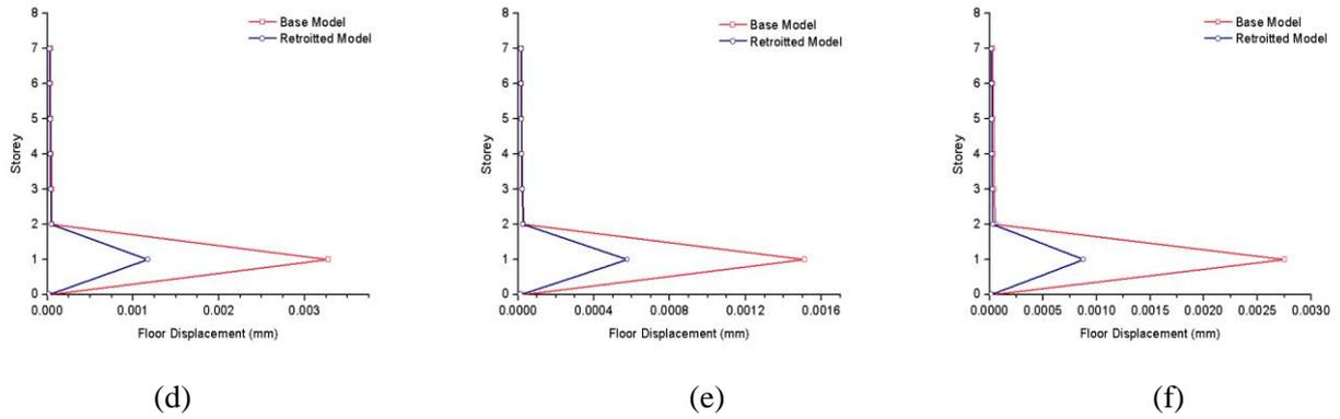
Fig. 13 - Observed values of Storey Drift for: (a) Chi-Chi, (b) El-Centro, (c) Kobe, (d) Landers, (e) Loma Prieta, and (f) Northridge
