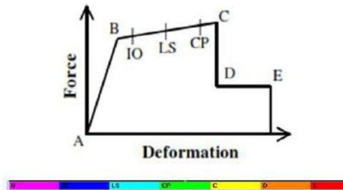
Fig. 7 - Force-Deformation for pushover analysis (Kiran et al, 2017)
