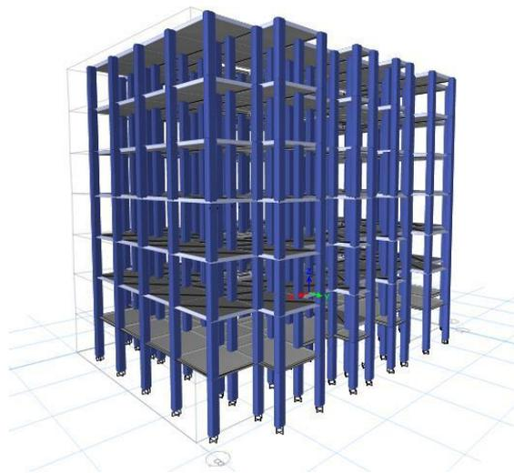
Fig. 4 - Parametric view of the Generated model (without infills)
