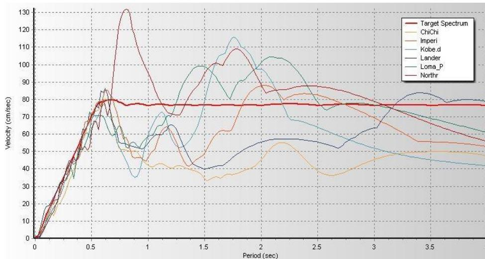
Fig. 6 - Scaled velocity time histories of considered earthquakes
