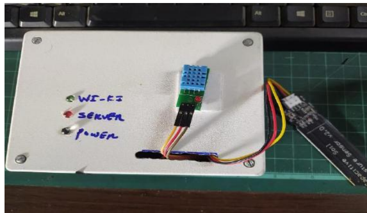
Figure 4. IoT Data Logger with DHT11 and Soil Moisture Level sensor
