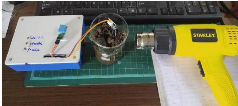
Figure 10. Iot data logger with external variable Temperature source by hot air gun
