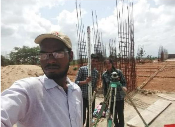
Fig.15(a) – Auto level & Levelling staff
