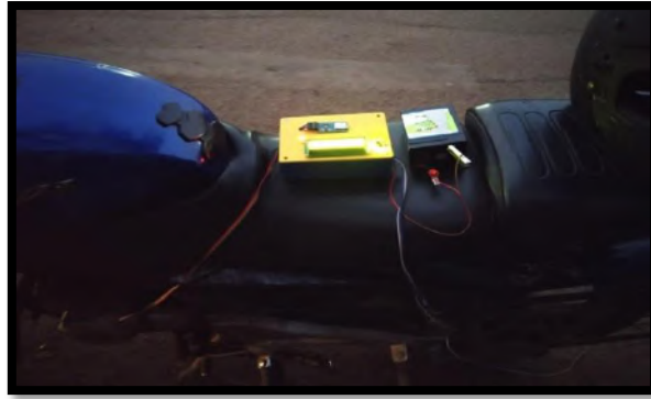
Fig 4.1: DATA Logger with battery powered placed on the two-wheeler
