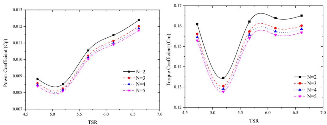
Figure 3. Effect of power and torque coefficient ( $C_p$ ) in variation of number of Savonius wind turbine as function of TSR ( $v= 5\text{m/s}$ ) (at  $N=500 - 700\text{rpm}$  and  $H=0.5\text{m}$ )
