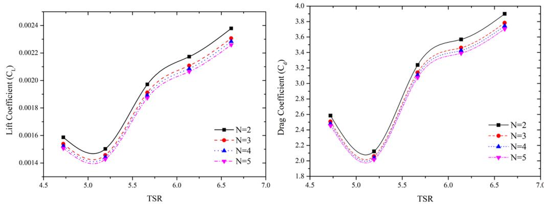
Figure 4. Effect of lift and drag coefficient ( $C_p$ ) in variation of number of Savonius wind turbine as function of TSR ( $v=5\text{m/s}$ ) (at  $N=500-700\text{rpm}$  and  $H=0.5\text{m}$ )
