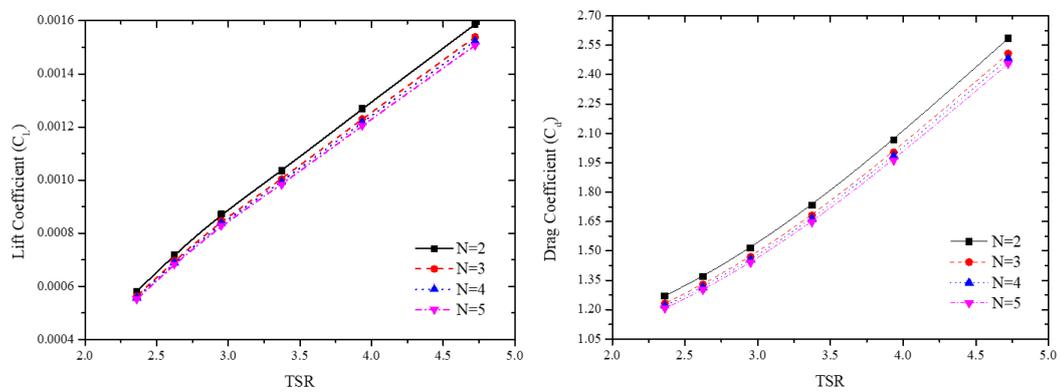
Figure 2. Effect of lift and drag Coefficient in number of Savonius wind turbine as function of TSR ( $v= 5 - 10\text{m/s}$ ) (at constant  $N=500\text{rpm}$  and  $H=0.5\text{m}$ )
