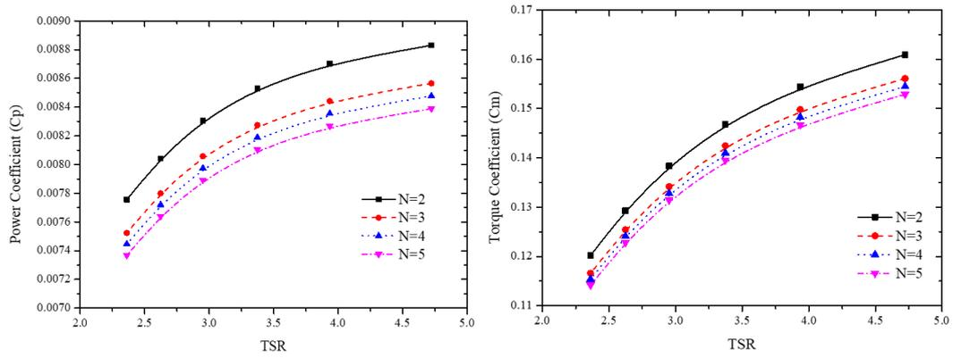
Figure 1. Effect of power and torque coefficient in variation of number of Savonius wind turbine as function of TSR ( $v= 5 - 10\text{m/s}$ ) (at constant  $N=500\text{rpm}$  and  $H=0.5\text{m}$ )
