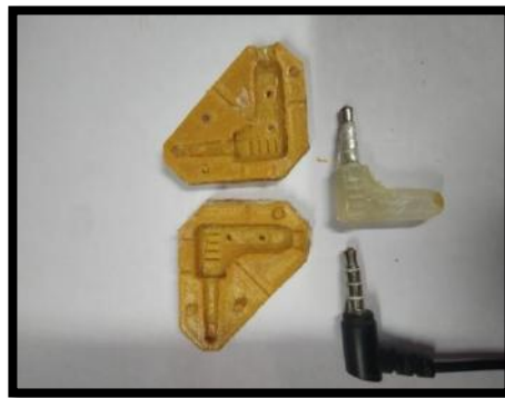
Figure 16. Closeup View Of 3D printed cast and Industrial Printed Cast
