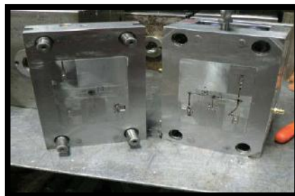
Figure 7. Standard two plates tooling – core and cavity are inserts in a mould base
