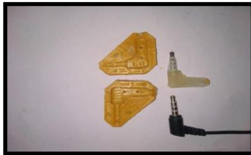
Figure 15. Observation Comparison Between 3D Printed Mould cast and Industrial Mould Cast
