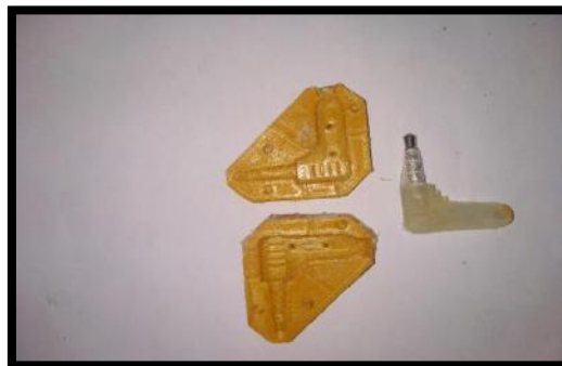
Figure 13. Taking Out The cast From 3D printed Mould
