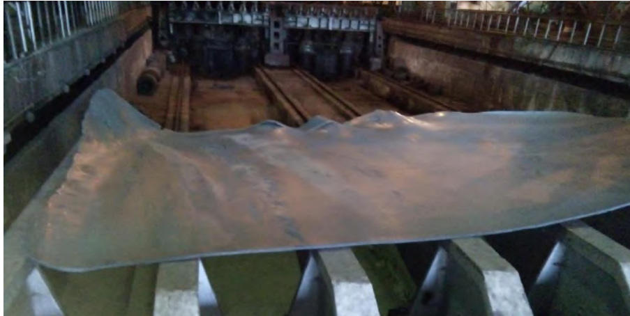
Figure 1. Edge Wave Defect in Steel Plate
