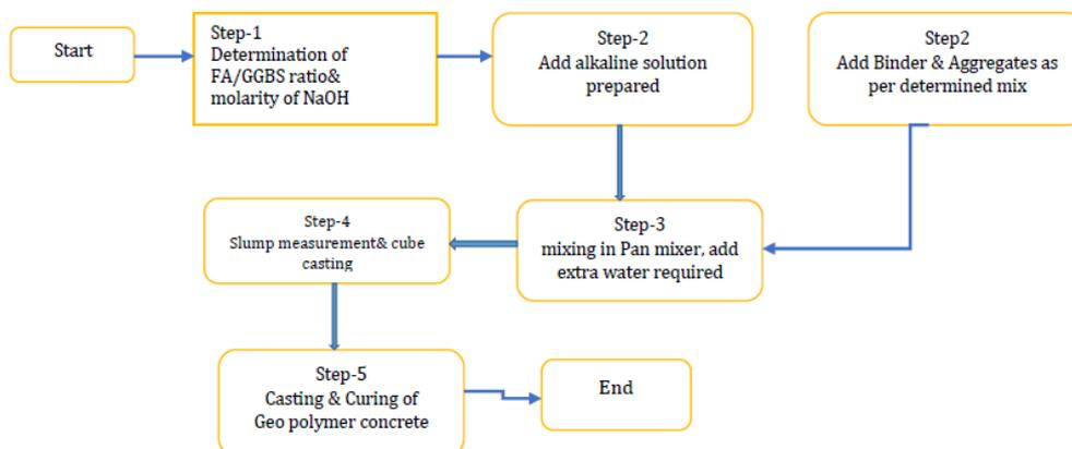
Figure1. Flow chart for the application of the mix design procedure.
