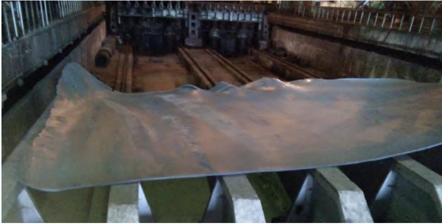
Figure 1. Edge Wave Defect in Steel Plate
