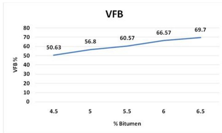
Figure 13. VFB of the samples with different proportion of bitumen
