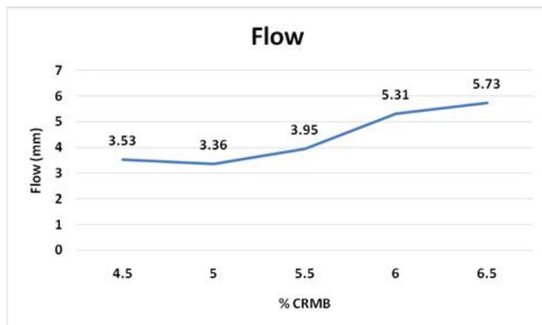
Figure 7. Flow value of the samples with different proportion of clean crumb rubber bitumen
