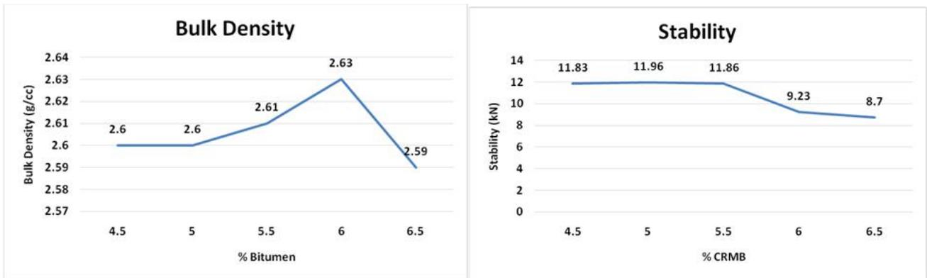
Figure 4. Bulk Density of the samples with different proportion of bitumen clean crumb rubber bitumen
