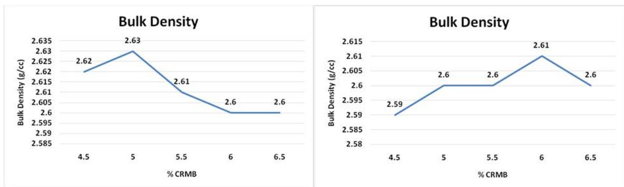
Figure 3. Bulk Density of the samples with different proportion of clean crumb rubber bitumen and unclean crumb rubber bitumen
