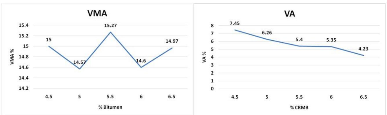
Figure 10. VMA of the samples with different proportion of bitumen and clean crumb rubber bitumen
