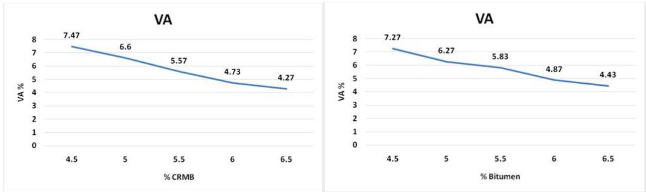
Figure 11. VA of the samples with different proportion of unclean crumb rubber bitumen
