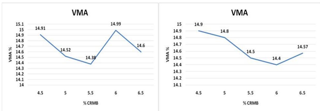
Figure 9. VMA of the samples with different proportion of clean crumb rubber bitumen and unclean crumb rubber bitumen
