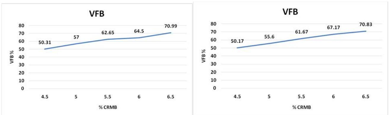
Figure 12. VFB of the samples with different proportion of clean crumb rubber bitumen and unclean crumb rubber bitumen
