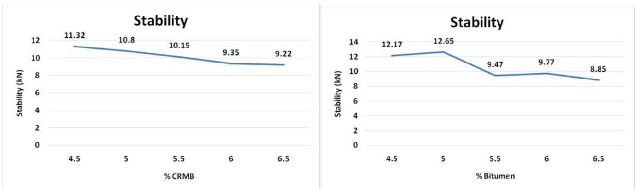
Figure 5. Stability of the samples with different proportion of unclean crumb rubber bitumen and Bulk Density of the samples with different proportion of bitumen
