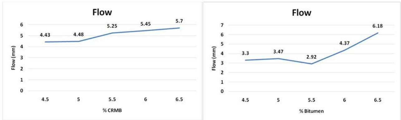
Figure 8. Flow value of the samples with different proportion of unclean crumb rubber bitumen and only bitumen
